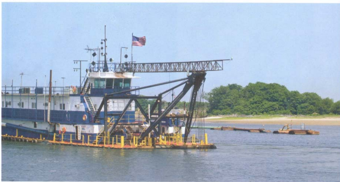
A working dredge displays a set of diamond shapes on the safe side for passing; you'll see ball shapes on the danger side.
