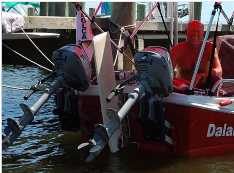
Dalamar’s twin air-cooled outboards. Of everything aboard his vessel, the outboards’ sheer pins are what fail most. Sheer pins are sacrificial pins mounted on the propeller. They are designed to
