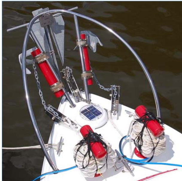
While Buzz prefers to stay in marinas, he has equipped "Dalamar" for anchoring out. Two Bruce anchors hang from the bow in twin anchor holders built from schedule 80 PVC pipe. Each anchor is attached to 150 feet of nylon anchor rode coiled on T-shaped PVC cleats. The third, Danforth anchor, lends holding power as required.
